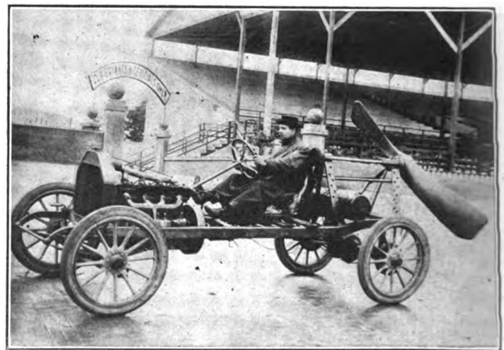
Overland "Wind Wagon," a cross between automobile and airplane, which covered five miles in 5:20
